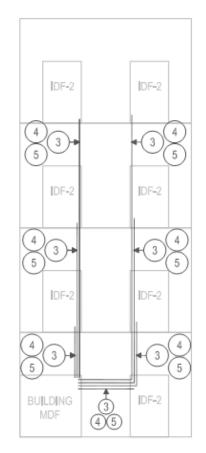
1) 24-STR 50 MICRON OM3 MULTI-MODE/12-STR 9 MICRON SINGLE MODE FIBER
