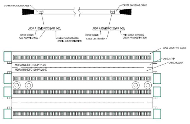
NOTE: 1) CABLE AND 110 BLOCK SHALL HAVE IDENTICAL LABEL AT BOTH ENDS
