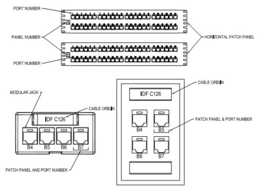
NOTE: 1) CABLE SHALL HAVE IDENTICAL LABEL AT BOTH ENDS 2) EACH PATCH PANEL SHALL BE UNIQUELY LABELED ALPHABETICALLY IN EACH MDF OR IDF
