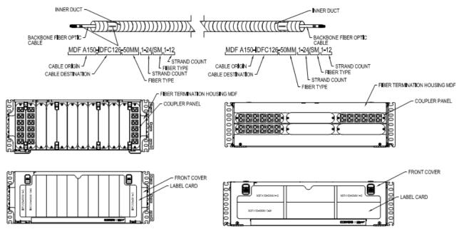
NOTE: 1) CABLE AND INNERDUCT SHALL HAVE IDENTICAL LABEL AT BOTH ENDS
