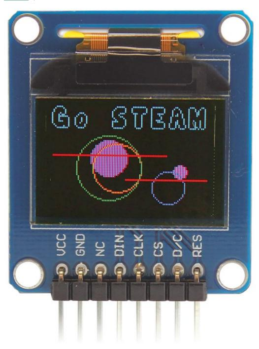
28087: 96 x 64 Color OLED Display Module - displaying text and shapes
