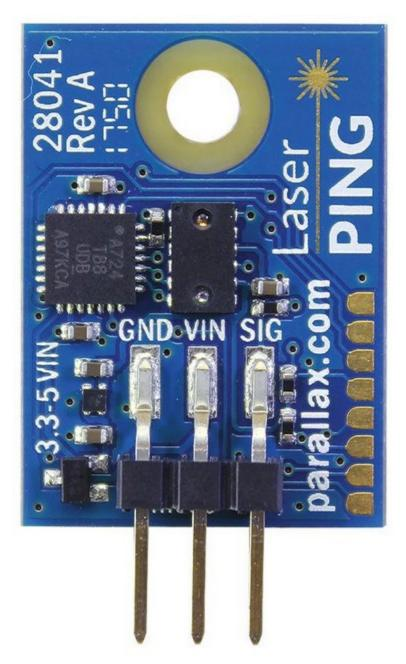
28041: LaserPING 2m Rangefinder - front view
