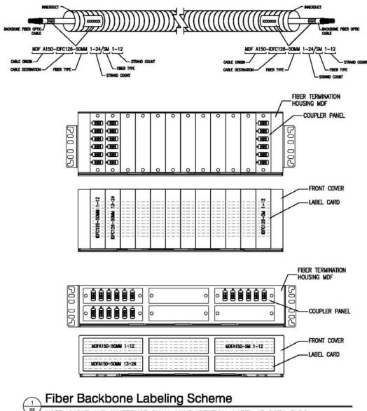
$\prime$  note: cable and innerduct shall have identical label at both ends
