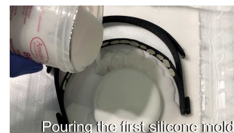
Pouring the first silicone mold
